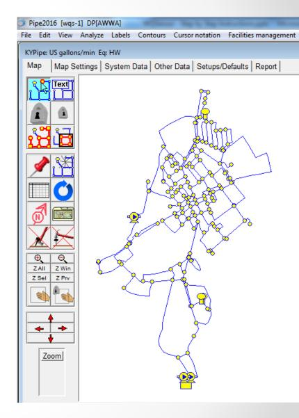
Press Shift-F7 key to launch optimal water quality sensor placement tool
